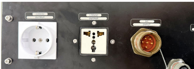
Detail – 220 VAC Schuko, 120 VAC universal socket and DC input connector
